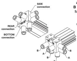
A = forward stroke connection B = backwards stroke connection M5 tube Ø4 and Ø6 fittings can be used for air connections. In case of use with 1600.16.01F mounting and REAR air connections use a 4mm pipe fitting.
