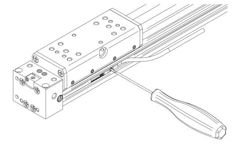
The two side slots allow the direct use of 1590....LRS... and LHS... sensors mounted from the top and positioned via the built in screw.
