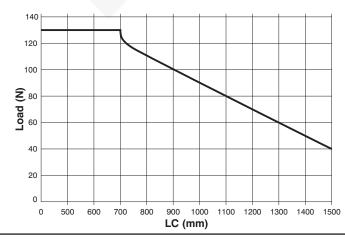
The graph shows the LC limit in conjunction with the applied load K beyond which it is necessaryto mount an intermediate side support in order to prevent the barrel from bending.
