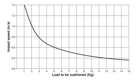
In case of extreme applications close to the maximum allowed values in the graph it is strongly recommended to ad external damping systems.
