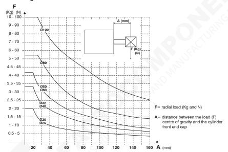
The diagram shows the maximum radial load F (in Newtons) that can be applied to the cylinder piston rod as a function of the distance A (in mm), based upon the standard version cylinder under static conditions.
