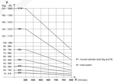
The diagram shows, for each diameter, the safety curves relative to the maximum loads which can be moved by the cylinder in function of it's speed V. The data has been calculated under the following test conditions: Cylinder mounted vertically with the rod pointing down, air pressure at 5 bar and with a guided load.
