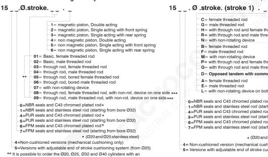
aluminium piston by replacing the '0' with 'K' in the ordering code. Example: 1540.20.10.01.1 (Acetyl Resin Piston) 1540.20.10.K1.1 (Aluminium Piston version)
