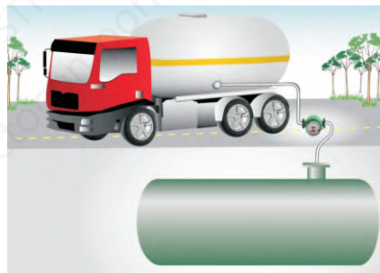
Fuel Oil transferring
