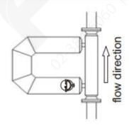
Flag installation—side mounted Generally, the Sensor is installed on the vertical pipeline to avoid the accumulation of particles in the measuring tube of the Sensor.
