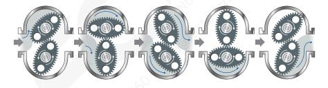
A conversion coefficient, specific to each meter size, enables the conversion of this frequency into a flow rate. The standard K factor depending on the meter size is available in the flowmeter's operating instructions, see Type \$077 \( \). To improve the measurement deviation, a device-specific K factor is given on the device label.
