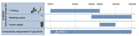
Note A: Only use plastic fitting in analytical variant with true union according to DIN 8063 (PVC), DIN 16962 (PP) or ISO 10931 (PVDF).
