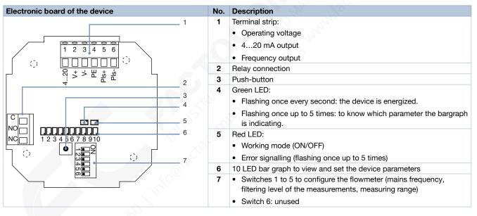
The device can be calibrated by means of the K-factor (conversion coefficient), or via the Teach-In function.
