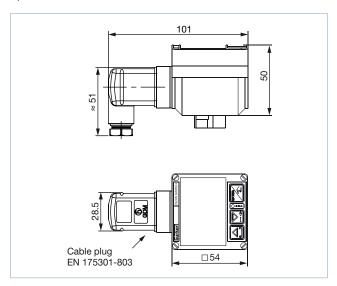
With Cable plug (EN 175301-803) and free positionable 5 pin M12 male fixed plug
