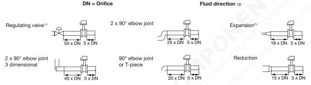
1.) If the valve cannot be mounted after the measuring device, the minimal distances have to be respected 2.) If an expansion cannot be avoided, the minimal distances have to be respected. Please note minimum flow velocity
