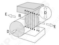
The signal voltage U is obtained by electrodes on both sides of the sensor and is proportional to the fluid flow rate and therefore the fluid flow rate. The signal is amplified, filtered and then accumulated, recorded and output.
