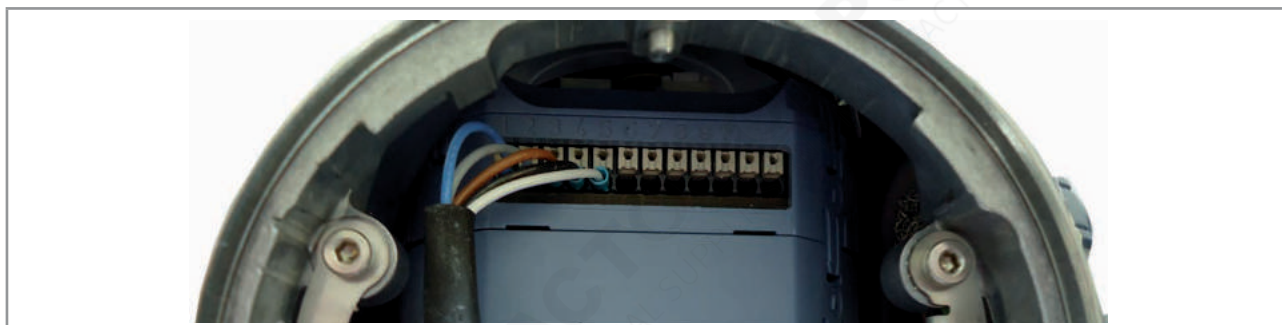
Fig. 24: Wiring of the 12 push-in terminal strip
