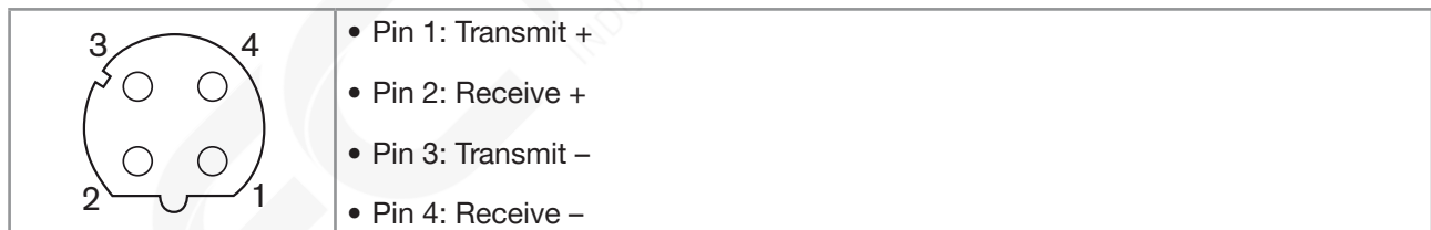
Fig. 36: Pin assignment of the 4-pin M12 female connector
