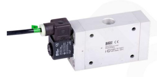
Electrically operated valves conform to equipment category 2 can be used in Zone 1 respectively in Zone 21. For the use in hazardous areas the category group of the used coil has to be taken into account. The specification of the whole equipment corresponds always to the lowest category of the single components.
